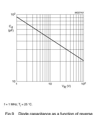
Fig.9 Diode capacitance as a function of reverse voltage; typical values.
